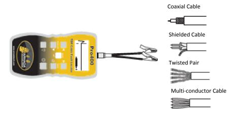
**Coaxial Cable:** Connect the red clip to the center wire and the black clip to the shield/screen.
